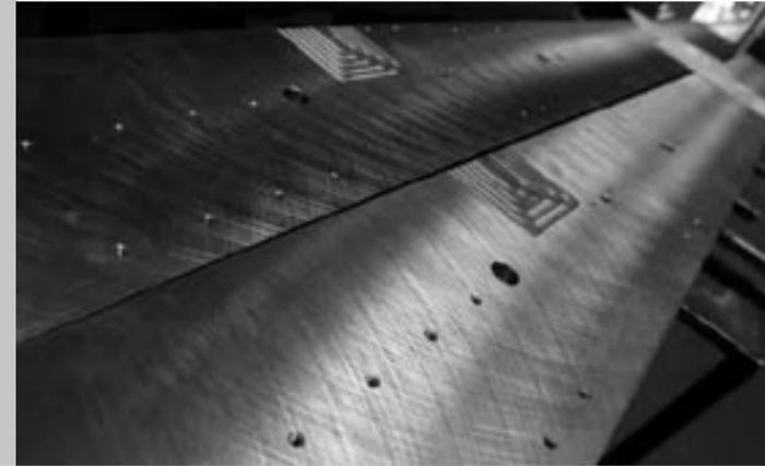
Our standard parallelism is 0.01 mm per meter, and the standard surface finish during fine grinding is  $Ra = 0.8 \mu\text{m}$ . Micro-precise guide rails are possible depending on the design.
