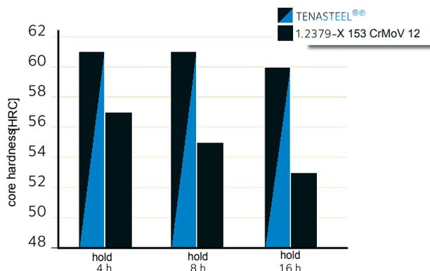
Please note that for nitriding treatment following hardening, it must be tempered at a minimum of 525°C.
