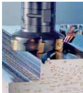
Entry via the "roll-in" method Wear after 800 machining passes.
